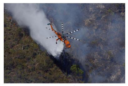
The Erickson Aircrane S-64E dropping fire suppressant foam' on a fire edge to support ground firefighting resources.
