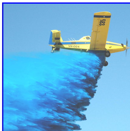
AirTractor 802 dropping thermogel fire suppressant. This blue colouring will be replaced with red/purple for the next fire danger season
