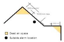
If a flat or sloping ceiling has closely spaced exposed beams the areas in between the beams should be considered as dead air space and the alarm should be attached to the bottom of a beam.
